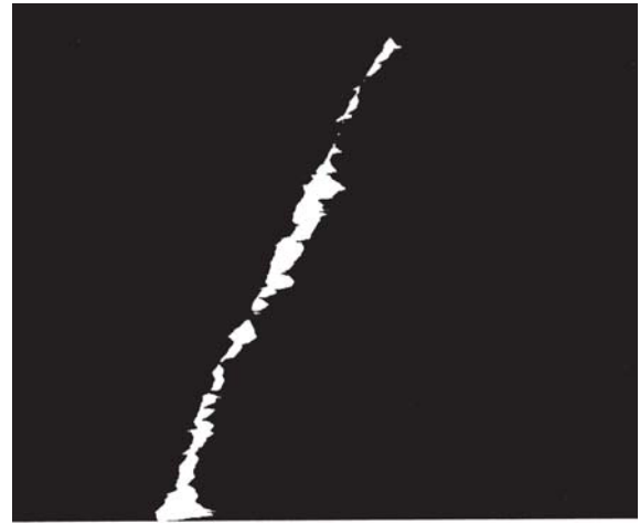
Fig. 13 Worn 6.350 mm small milling cutter after 5 machining passes. Average wear, 1.5 \times 10^{-2} mm; maximum wear, 2.54 \times 10^{-2} mm
