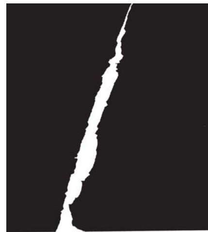
Fig. 15 Worn 6.350 mm small milling cutter after 15 machining passes. Average wear, 3.30 \times 10^{-2} mm; maximum wear, 9.14 \times 10^{-2} mm
