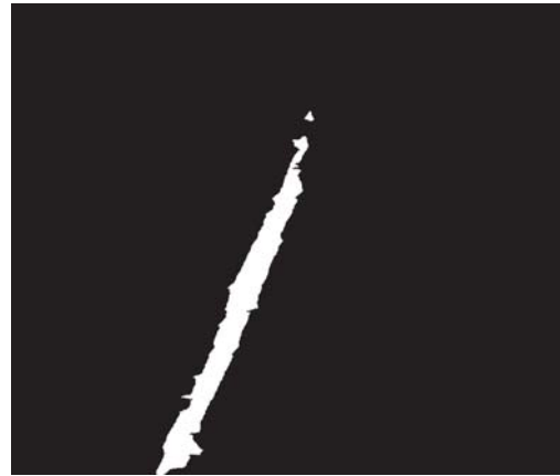
Fig. 18 Worn 9.525 mm small milling cutter after 30 machining passes. Average wear, 3.30 \times 10^{-2} mm; maximum wear, 6.10 \times 10^{-2} mm
