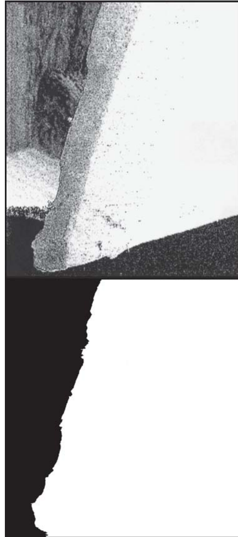
Fig. 8 Worn 6.350 mm small milling cutter after 15 machining passes
