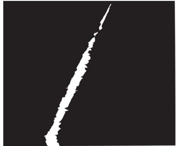
Fig. 14 Worn 6.350 mm small milling cutter after 10 machining passes. Average wear, 2.45 \times 10^{-2} mm; maximum wear, 4.83 \times 10^{-2} mm
